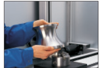
Simply put the roll on the plug – either manually, by fork lifter or crane
