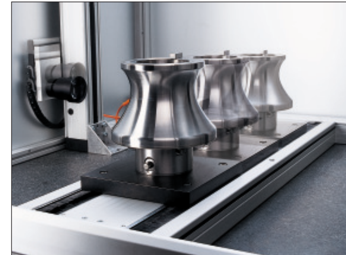
Scanning the roll between a CCD camera and a background illumination
